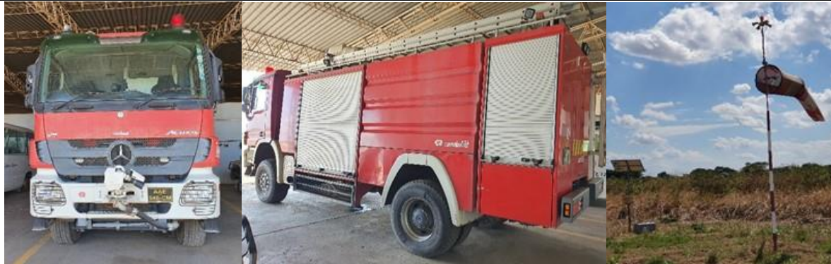
From left to right: Firefighting 6.000 litres capacity vehicle – Rosenbauer (left and centre) and anemometer (right)
