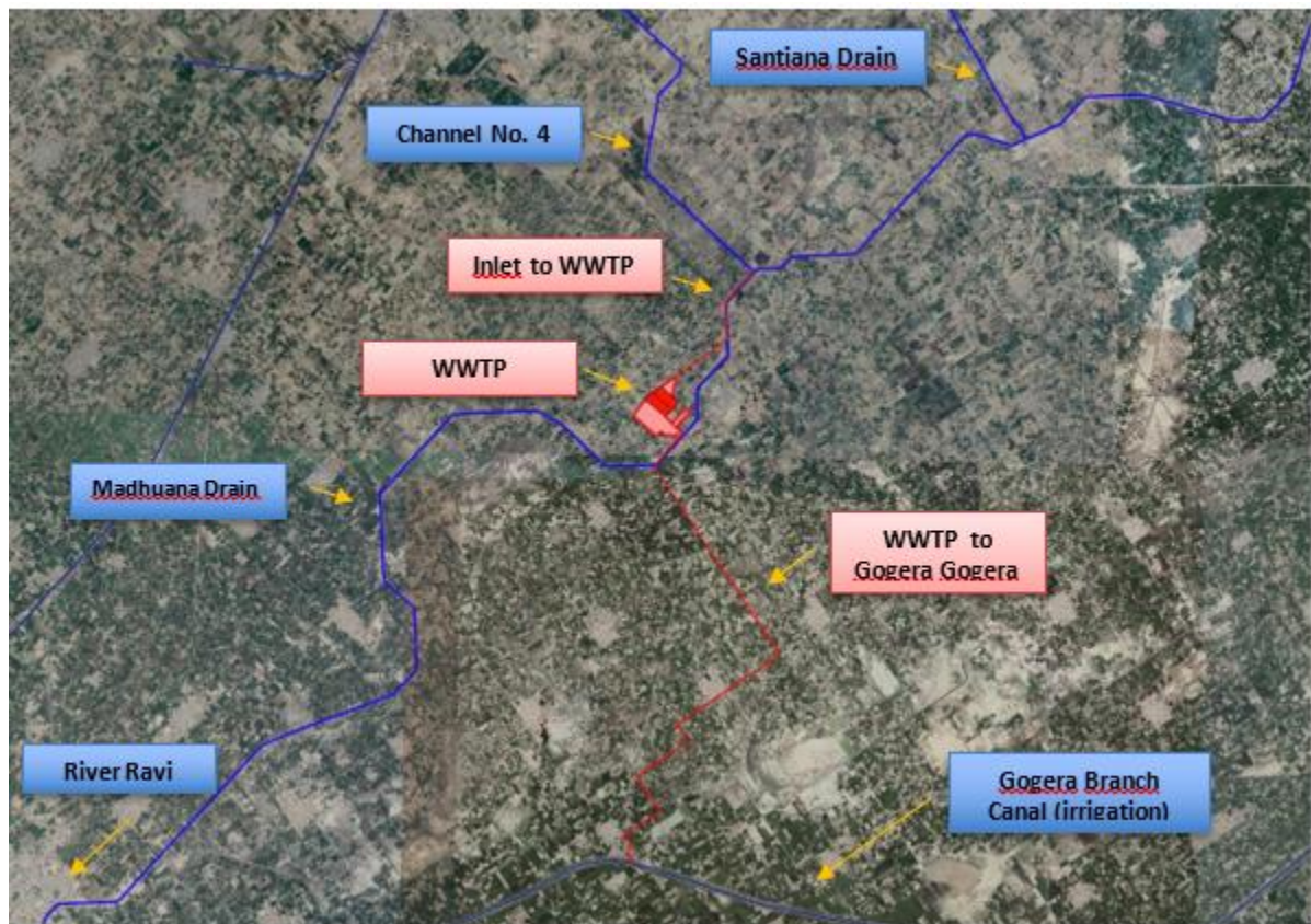
Overview drawing of WWTP and new pipelines (illustrated in red) and existing drainage channels (blue) in East Faisalabad.
